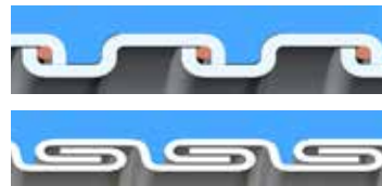
Square-Locked Design with integral bonding wire 1/2" - 1-1/4"
