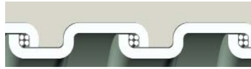
Square-Locked Design with cord packing 5/16" through 1-1/4"
